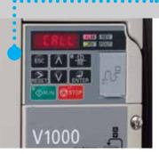
Stirrer rotation inverter, range from 7 up to 70 Hertz. With the new Smarty TTi a perfect batch freezing depending on the produced quantities and features of the mix and on the ingredients and their mix formulation, is now readily available thanks to PLC and inverter. Totally new is the possibility to select the automatic speed adjustment mode of the outgoing gelato, which does not melt during the whole outgoing process.
