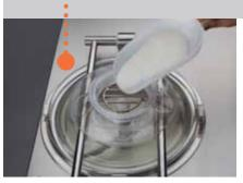
Double lid with opening system actuated by servo-assisted hydraulic pistons for easy ingredient introduction even in case of product in progress. The machine has not to be stopped in full compliance with certified EC safety regulations.
