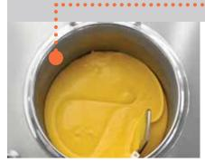
The bain-marie cooling and storage system of the latest generation guarantees temperature uniformity and control without thermal inertia. Ice-prevention system for min. processed quantities and during storage.
