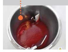
Chef Cream TTi manages and controls by means of a dedicated programme temperature progression in time and speed according to the product in progress. This avoids the unpleasant effect of uncontrolled mass volume increase and consequent overflow due to excessive heating. Quantities at full load are therefore optimized for each product.
