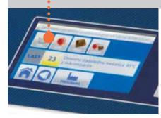
Innovative PLC system that controls the numerous programmes of Chef Cream TTi, many of which are customizable. The wide LCD-display shows in detail the step to be performed for each procedure.
